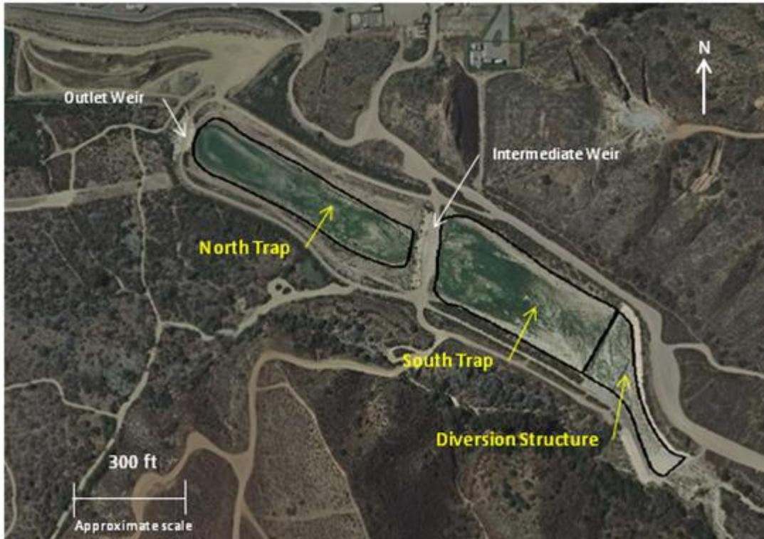
Figure C3. Sediment traps at the mouth of Goat Canyon and areas used for analysis (Google Earth).
